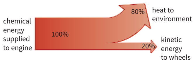
Figure 5.16 We want a car engine to supply kinetic energy. This Sankey diagram shows that only 20% of the energy supplied to the engine ends up as kinetic energy – it is 20% efficient.
