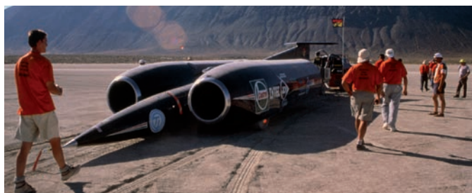
Figure 3.7 The Thrust SSC rocket car broke the world land-speed record in 1997. It achieved a top speed of 763 mph (just over 340 \text{ m s}^{-1} ) over a distance of 1 mile (1.6 km).
