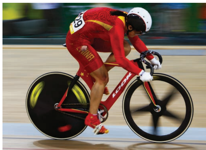
Figure 3.11 A racing cyclist adopts a posture which helps to reduce drag. Clothing, helmet and even the cycle itself are designed to allow them to go as fast as possible.
